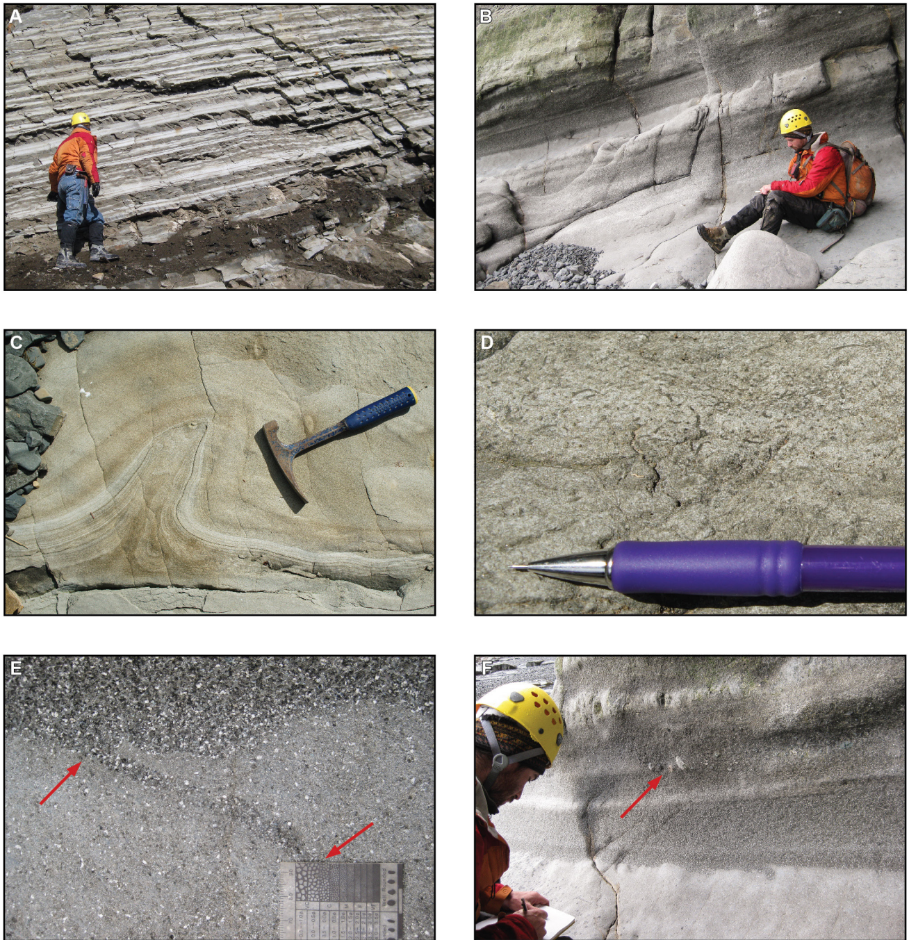
Figure 12. Photographs exhibiting outcrop and lithologic characteristics of the lower sandstone member, Naknek Formation. (A) Typical exposure of color-striped (gray- and brown-weathering), thin- to medium-bedded, tabular, arkosic, very-fine- to fine-grained sandstone beds along Oil Bay's west shore. Geologist for scale. (B) Outcrop of medium- to very-thick-bedded, medium- to coarse-grained sandstone beds that are structureless to faintly stratified and pervasively bioturbated. (C) Convolute laminations are commonly observed in fine-grained sandstone beds of the lower sandstone member. Hammer is 31 cm long. (D) Discrete trace fossils are present throughout much of the lower sandstone member; curvilinear, siltstone-filled tubes hosted in very-fine-grained sandstone immediately above pencil are probable Phycosiphon . Pencil above rubberized grip is 1 cm diameter. (E) A very-coarse-grained sandstone overlying medium-grained sandstone. A burrow (between red arrows) records bioturbation, and "floating" very-coarse sand grains in the medium-grained sandstone yield a "bimodal" texture that is further suggestive of syndepositional biogenic activity. Scale on left of grain-size card in mm. (F) Pebbles (red arrow) in the coarse sandstone facies of the lower sandstone member; gravel-sized clasts are rarely observed in the lower sandstone. Geologist for scale. Photographs by T.M. Herriott.
