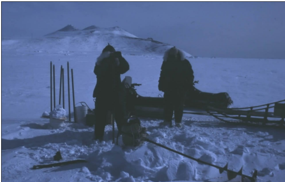
Figure 2A and 2B. Sampling the seafloor with a split Shelby tube sampler and screw-on extension pipes; water depth approximately 10 m. Pressure ridge in background marks edge of shorefast ice and western edge of Prince of Wales Shoal; sample 43, near the pressure ridge in photo, was at 23 m depth.
