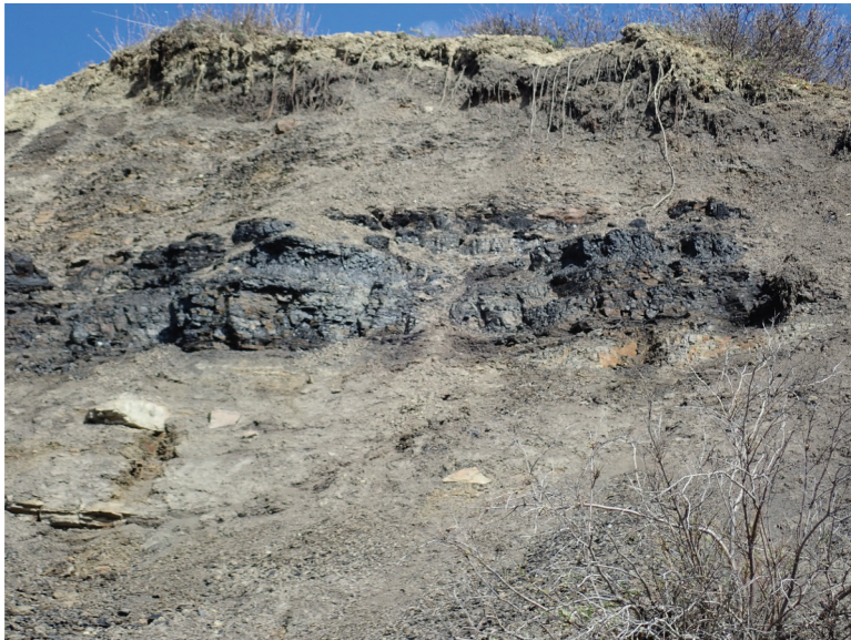
Figure 4. Lower coal interval sampled (18NH008-2). Coal bed is one meter thick.
